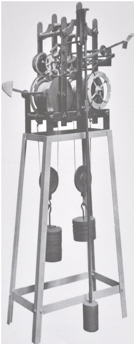
Two-Train Turret Movement East Bergholt Church, 1764 (BM Collection No. 113, p146)
