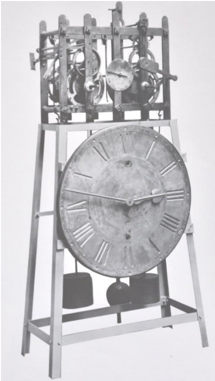
Two Train Turret Movement from St Nicholas Church Colchester 1767 (BM Collection No. 99, p148)
